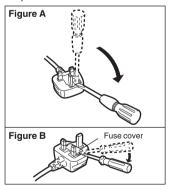
2. Replace the fuse and close or attach the fuse cover.
